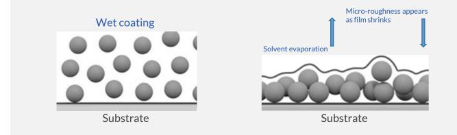
After the paint film dries, the dispersed matting agent particles within the applied film create a micro-roughening of the surface and film shrinkage occurs
